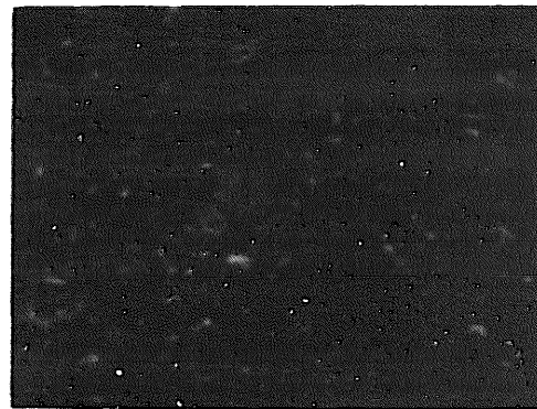
Figure 1-13. Small bright spots caused by minute imperfections in storage mesh
